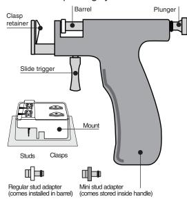
When you first receive your instrument, the regular adapter is already in the plunger of the instrument. If you are piercing with a Mini stud, you must remove the regular adapter and install the Mini adapter (stored in the handle of the instrument).
